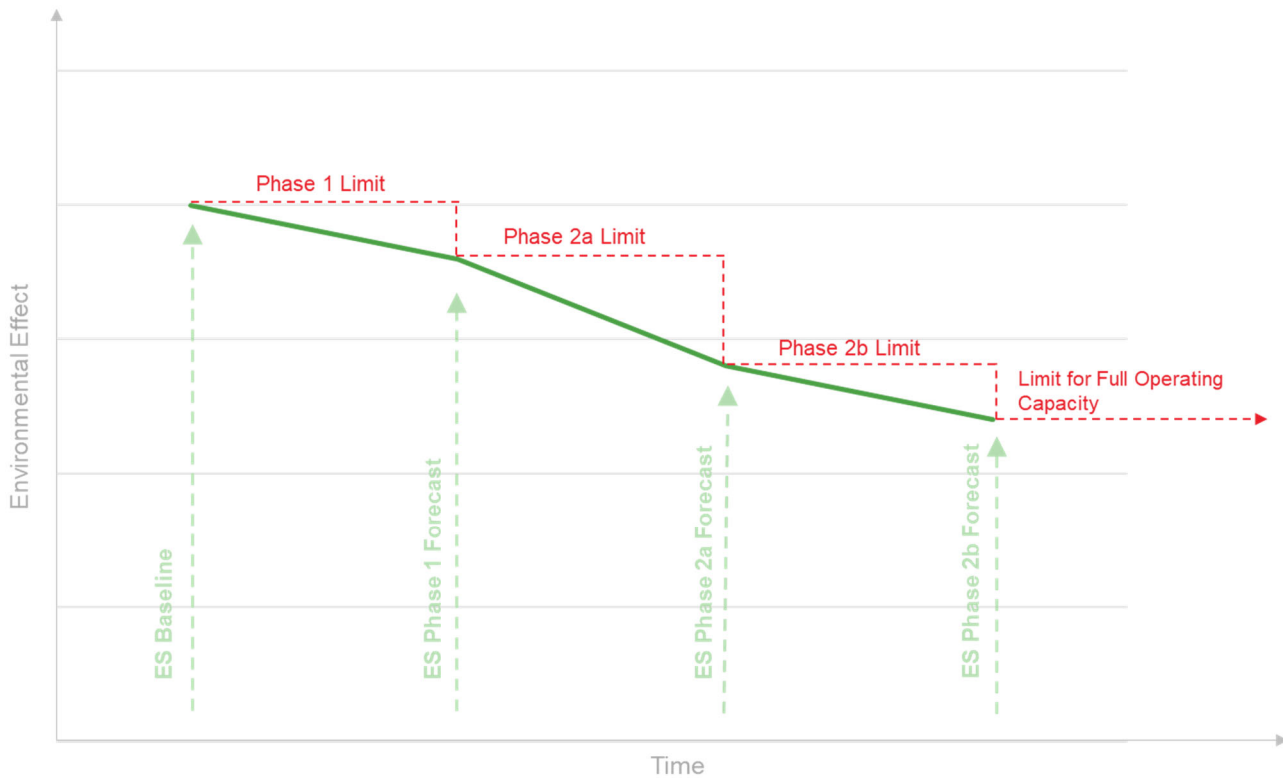
Figure 3.2: Conceptual approach to setting of Limits between Phases where environmental effects decrease over time
